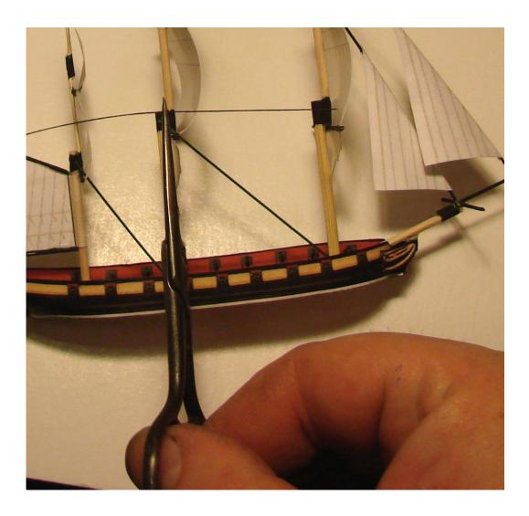
If you're not certain that a cut piece will fit where it is intended to go, it's a good idea to "dry fit" it in place without any glue, to check the length. It is much easier to trim it now than it will be after it is glued in place.
