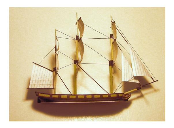
The next group of rigging to add is the shrouds and backstays, which run from the channels along the sides of the ship, up to the mastheads. As before, hold a piece of rigging material up to the model in the place it belongs, and cut it with the scissors.
