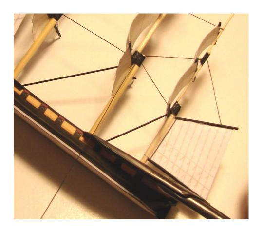
When there are multiple pieces of rigging going in the same place, as with the shrouds, use one of the pieces as a template to measure and cut as many as you will need. In this case, I will be placing four shrouds on each side of the mast, for a total of eight.
