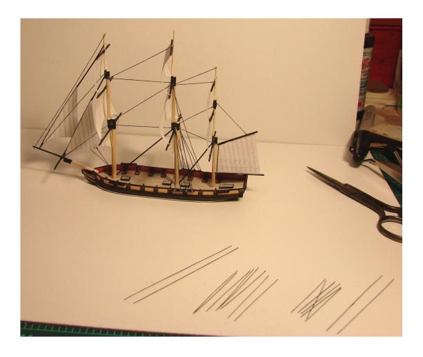
Here the model has all of the shrouds and backstays in place. Laid out on the board are the pieces for the next group of rigging to be added; the braces. Braces run from the ends of the yards, usually to the heads of the next mast. A pair will be needed for each yard.
